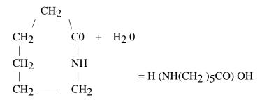
Nylons are among the toughest of all thermoplastics with excellent chemical, abrasion and creep resistance. This, together with high tensile strength, rigidity and heat distortion temperatures, makes nylon a very popular, cost effective, engineering resin.
