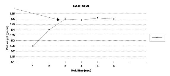
Cavity pressure readings taken near the gate can also be used to determine ideal screw forward time. A sharp drop in pressure as injection time concludes may indicate the gate has not been sealed properly and discharge has occurred.
